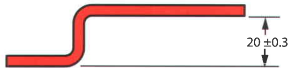
Directly toleranced (plus/minus) dimension
